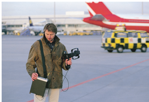
Miniport Receiver EB200 with active handheld directional antenna for portable radiolocation in frequency range 10 kHz to 3 GHz
