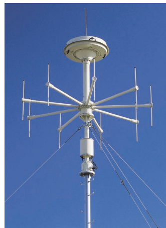
Fig. 16: Direction Finder DDF06M (photo 42136) operating on the principle of a correlation interferometer for the frequency range 20 MHz to 3000 MHz. Nine antenna elements are used for each of the three frequency subranges (photo 43073_2)
